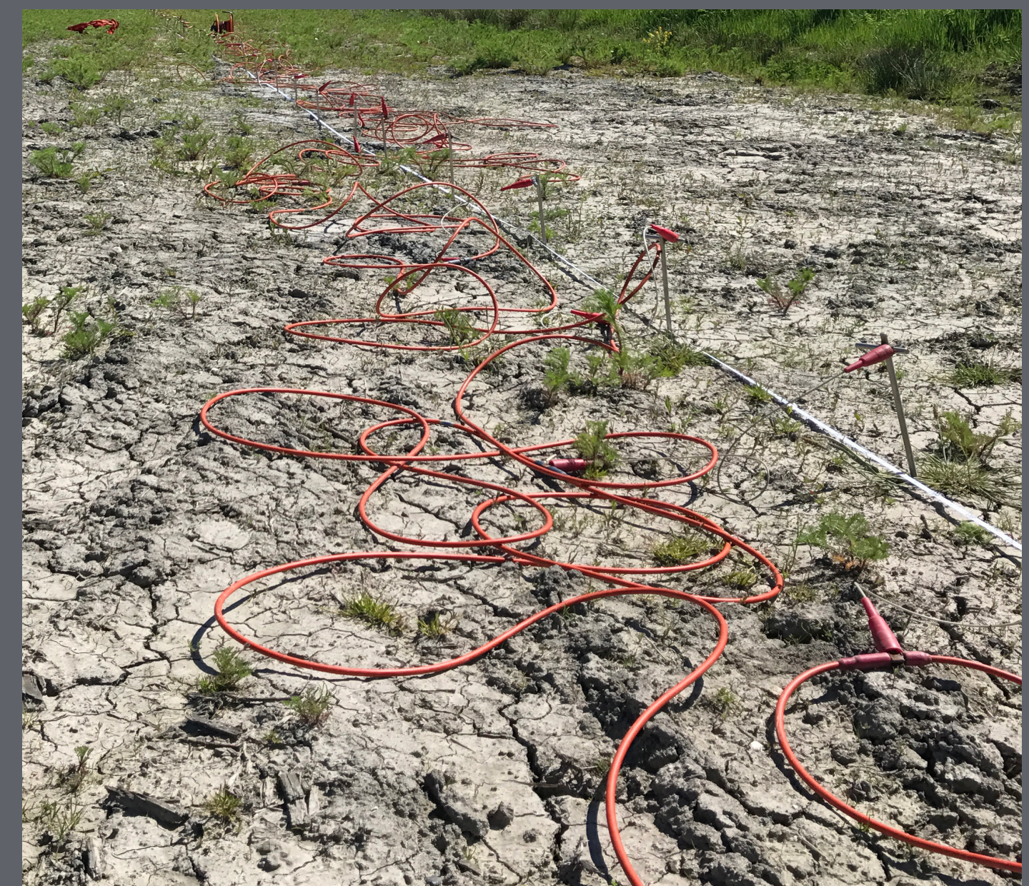
Electrical Resistivity Tomography
