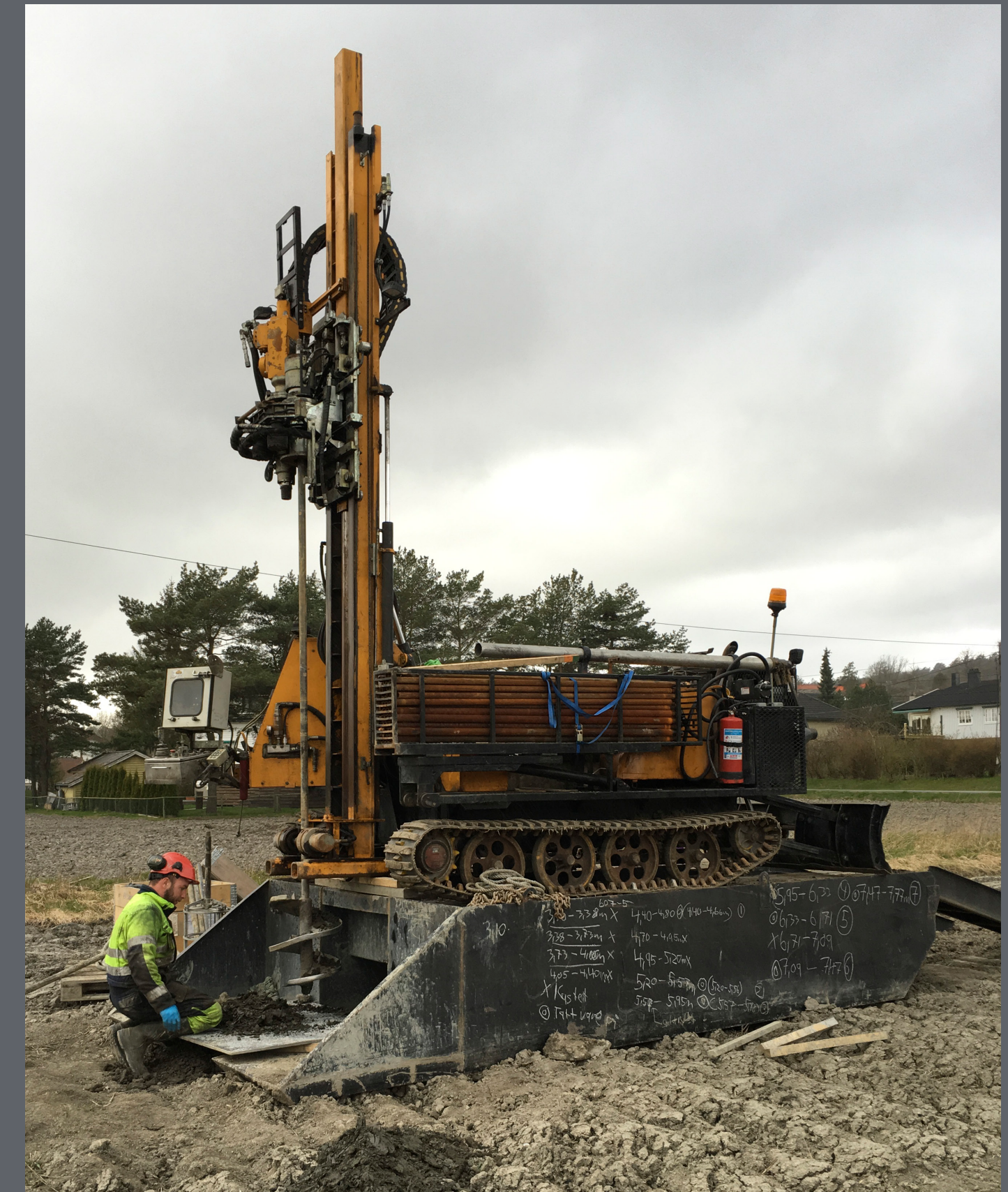
Block sampling to obtain high quality soil samples
